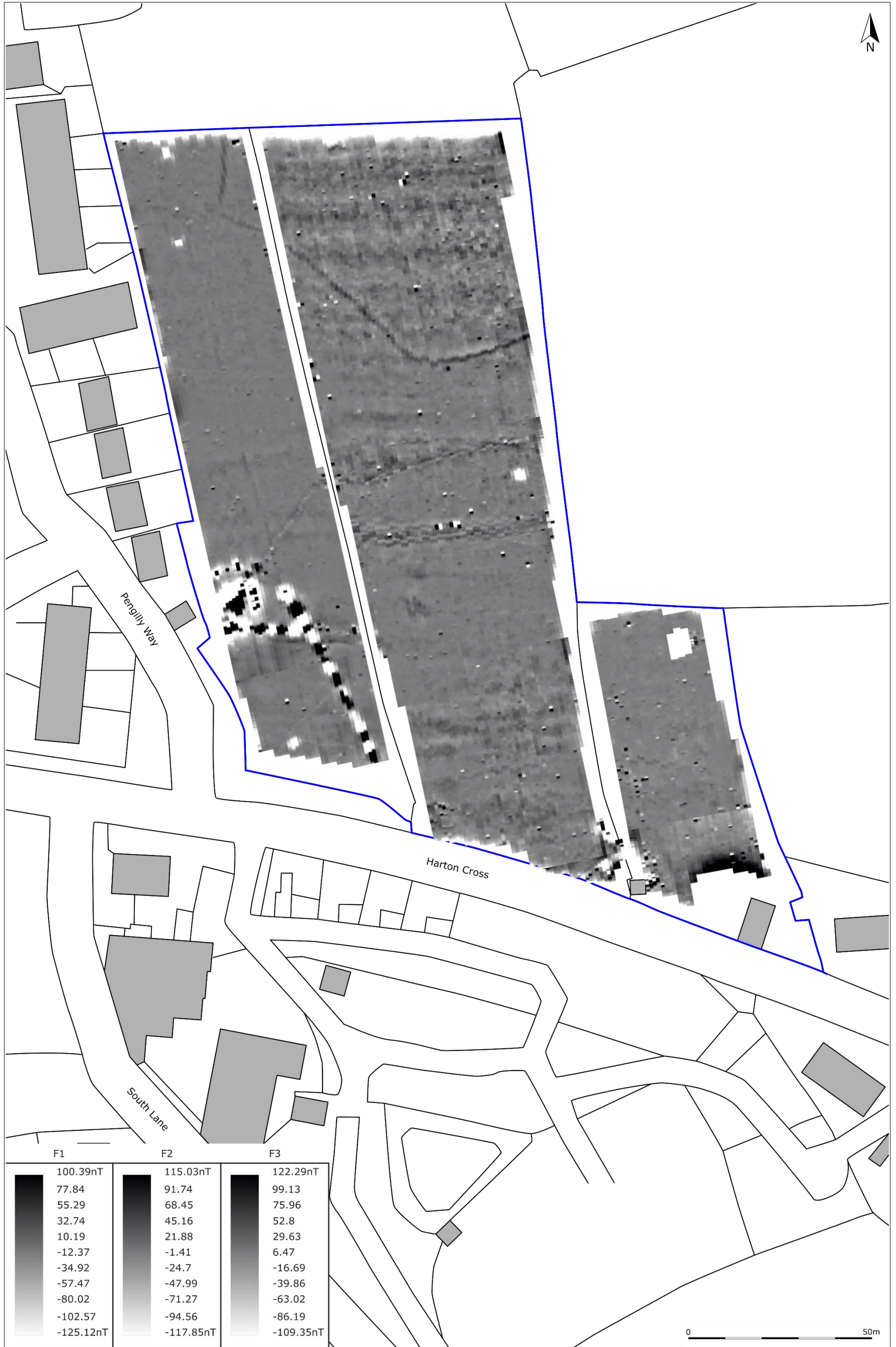
2. SHADE PLOT OF GRADIOMETER SURVEY DATA; MINIMAL PROCESSING.
