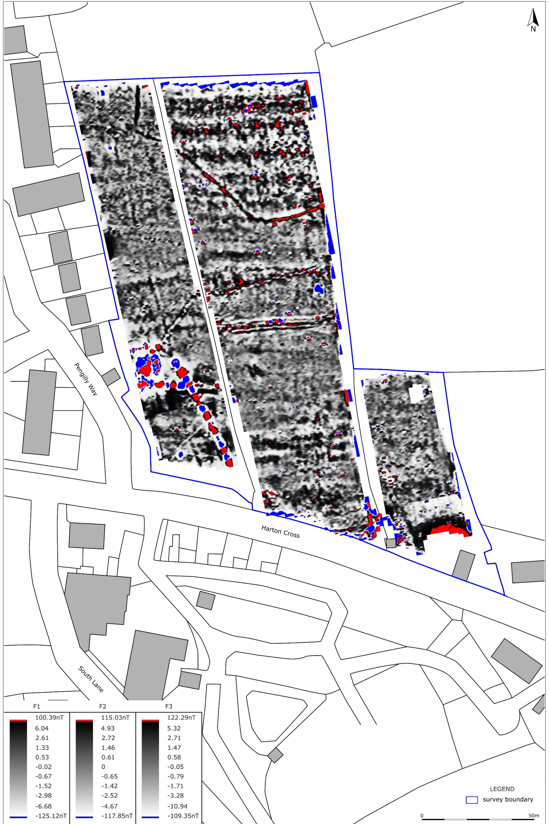
3. RED-GREY-BLUE SHADE PLOT OF GRADIOMETER SURVEY DATA; BAND WEIGHT EQUALIZED, GRADIATED SHADING.
