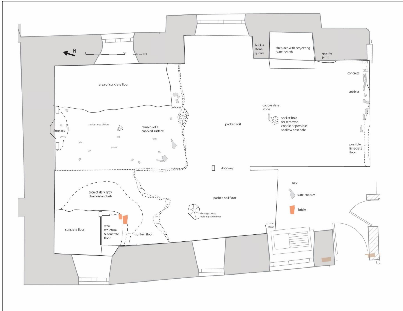
FIGURE 11: ANNOTATED PLAN OF THE FLOOR, IN FORMER NO.2, THE OLD CLERGY HOUSE, OVERLAID ON THE ARCHITECTS PLANS (AS SUPPLIED BY CLIENT), SHOWING THE LOCATIONS OF THE REMAINING COBBLES.
