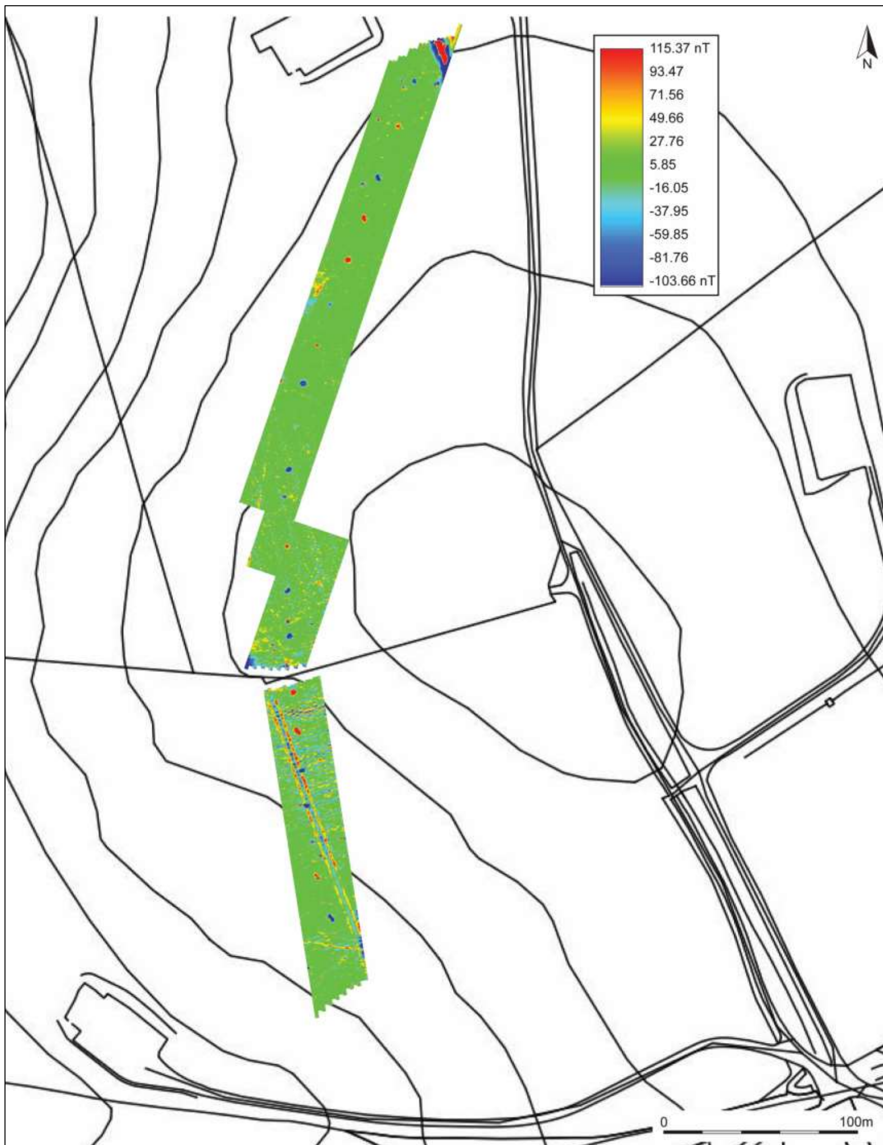
FIGURE 7: RED-BLUE-GREEN(2) SHADE PLOT OF GRADIOMETER SURVEY DATA; GRADIATED SHADING.
