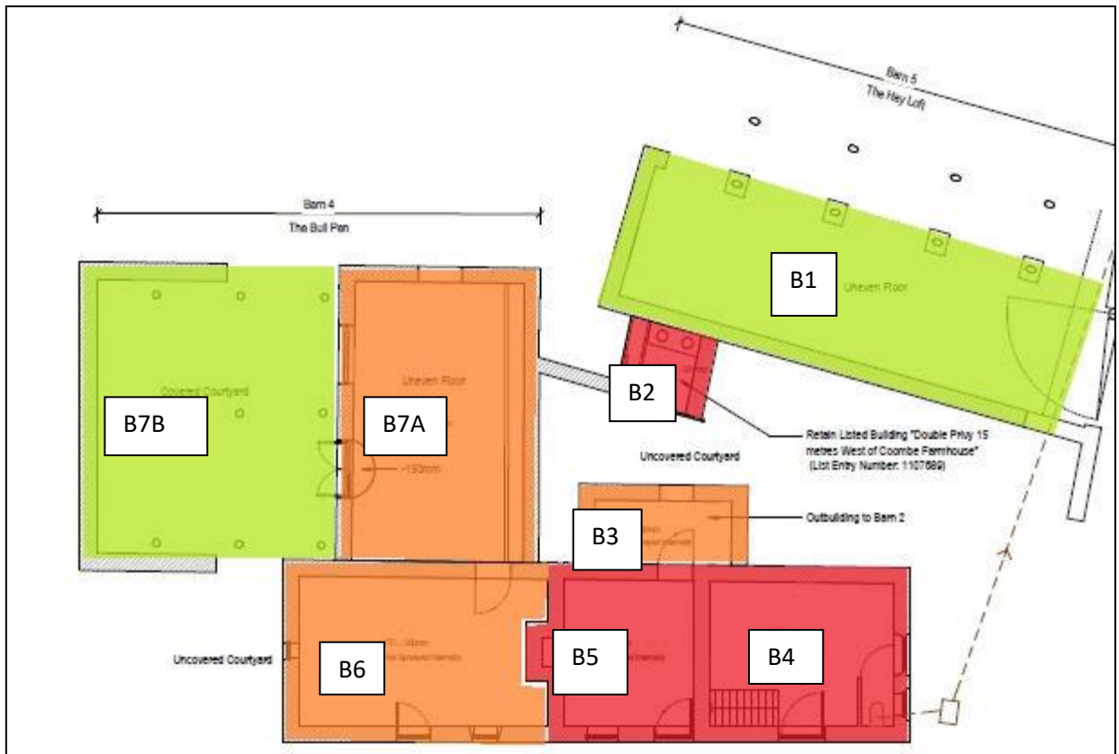
FIGURE 33: GROUND FLOOR PLAN OF THE BARNs SHOWING LEVELS OF SENSITIVITY TO CHANGE; ANNOTATED FROM PLANS AS SUPPLIED BY AGENT.
