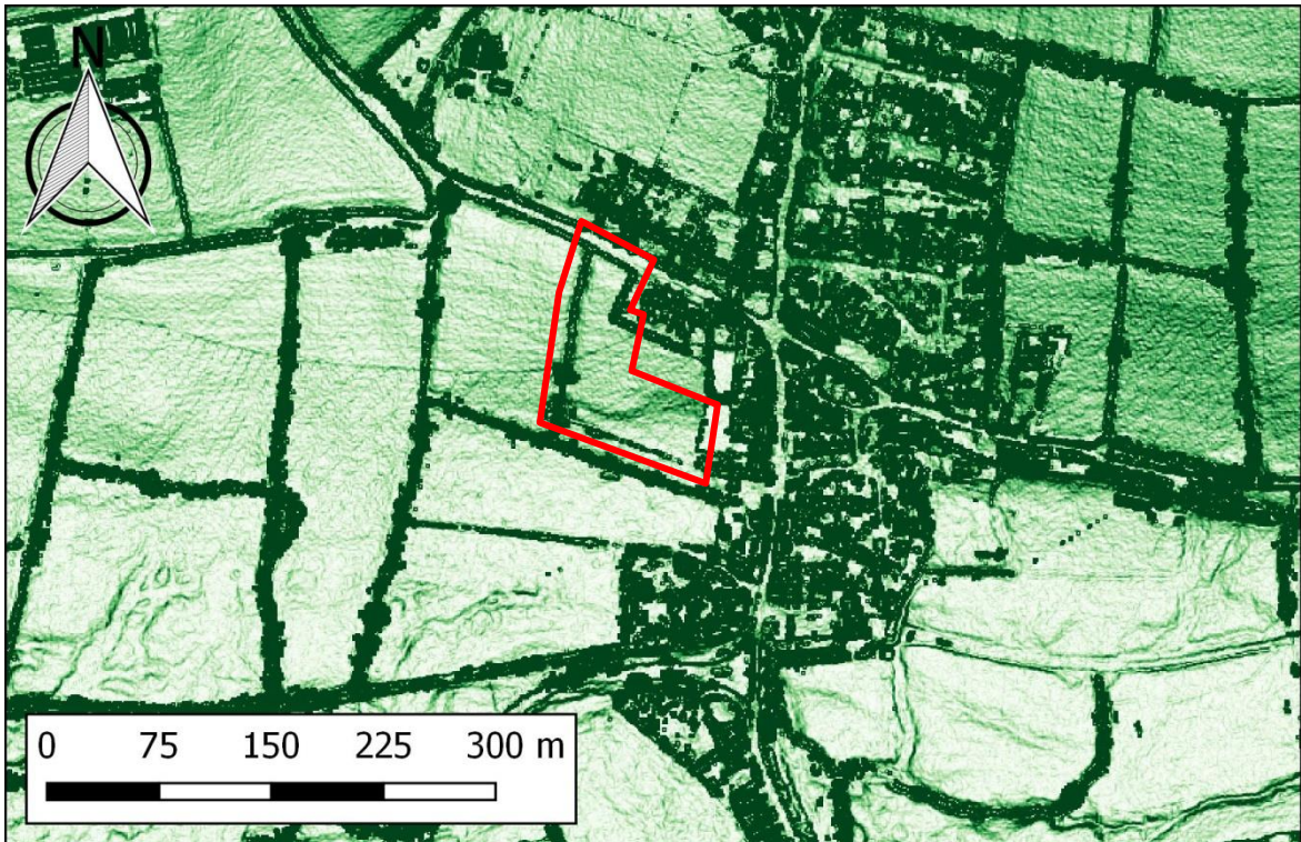
FIGURE 6: IMAGE DERIVED FROM ENVIRONMENT AGENCY LIDAR DATA (THE SITE IS INDICATED). PROCESSED USING QGIS VER2.8.1 TERRAIN ANALYSIS (SLOPE). CONTAINS FREELY AVAILABLE LIDAR DATA SUPPLIED BY NATURAL ENVIRONMENT RESEARCH COUNCIL (CENTRE FOR ECOLOGY & HYDROLOGY; BRITISH ANTARCTIC SURVEY; BRITISH GEOLOGICAL SURVEY); ©NERC.
