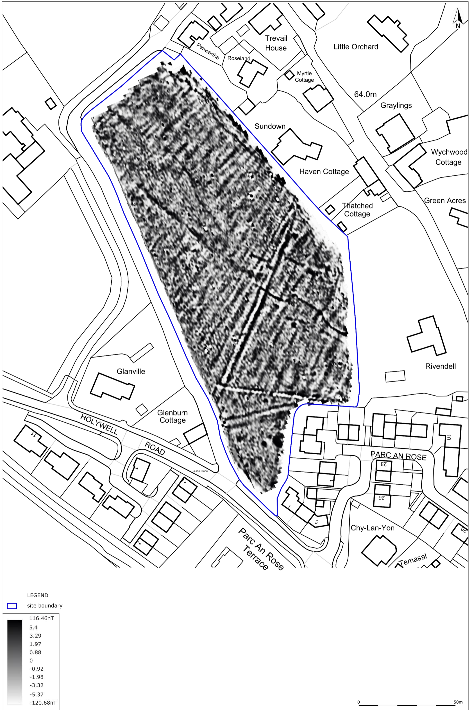
FIGURE 9: SHADE PLOT OF THE GRADIOMETER SURVEY DATA; BAND WEIGHT EQUALIZED, GRADIATED SHADING.
