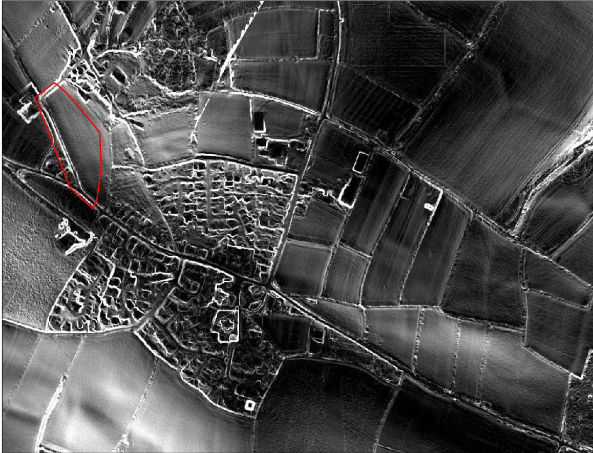
FIGURE 8: IMAGE DERIVED FROM LIDAR DATA (PROCESSED USING QGIS VER2.18.4, TERRAIN ANALYSIS/SLOPE, VERTICAL EXAGGERATION 3.0). DATA: CONTAINS FREELY AVAILABLE DATA SUPPLIED BY NATURAL ENVIRONMENT RESEARCH COUNCIL (CENTRE FOR ECOLOGY & HYDROLOGY; BRITISH ANTARCTIC SURVEY; BRITISH GEOLOGICAL SURVEY); ©NERC (CENTRE FOR ECOLOGY & HYDROLOGY; BRITISH ANTARCTIC SURVEY; BRITISH GEOLOGICAL SURVEY) 2018.
