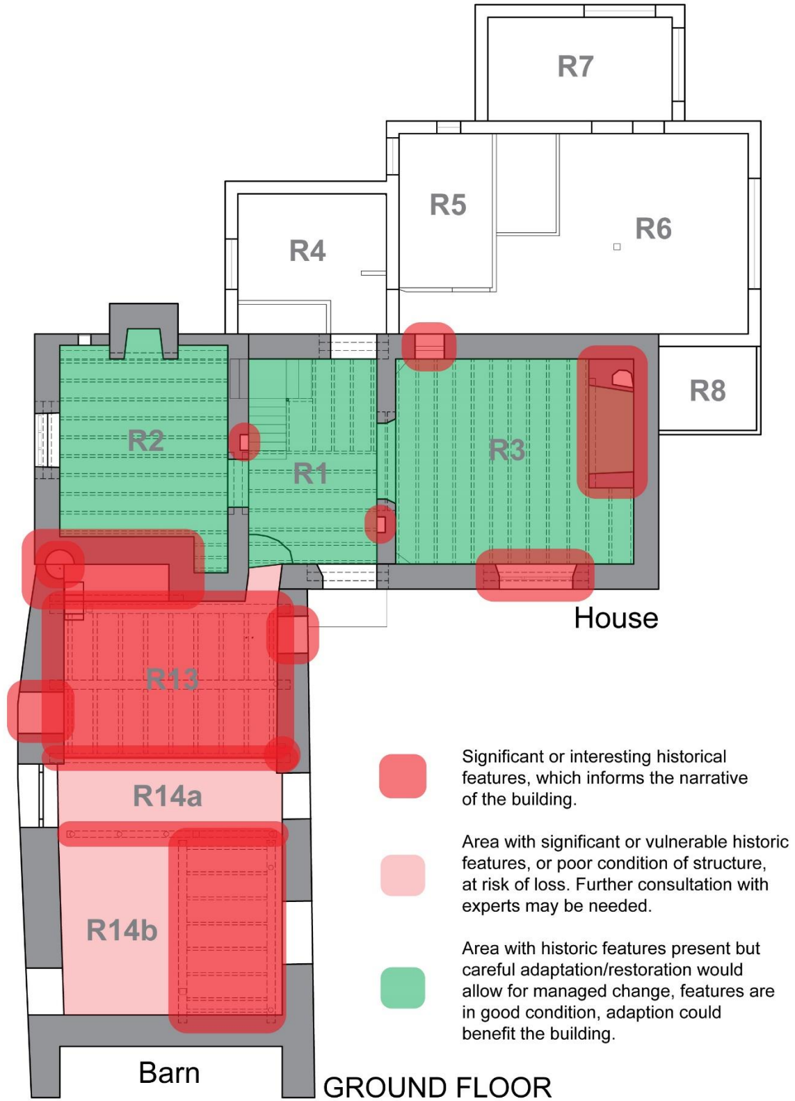
FIGURE 24: GROUND-FLOOR PLANS, SHOWING THE LOCATION OF SIGNIFICANT FEATURES AND SENSITIVITY OF SPACES (BASE PLAN PRODUCED BY THE CLIENT).
