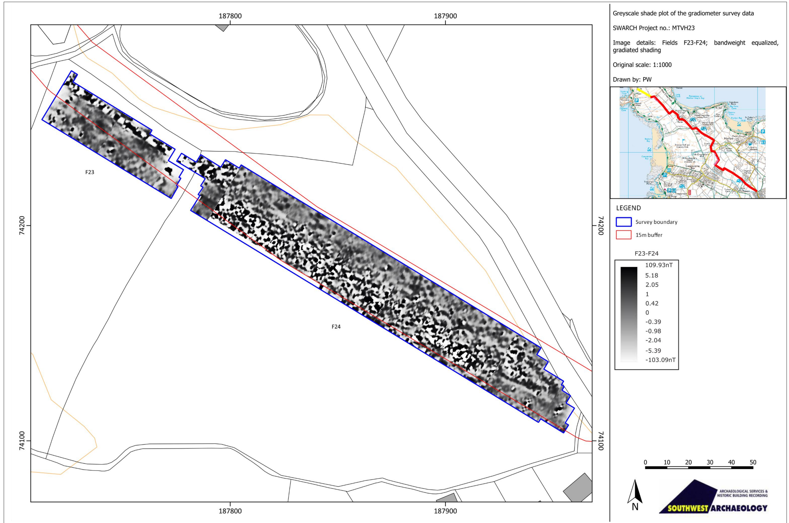
7. GREYSCALE SHADE PLOT OF GRADIOMETER SURVEY DATA (FIELDS F23-F24); BANDWEIGHT EQUALIZED, GRADIATED SHADING (CONTAINS ORDNANCE SURVEY DATA © CROWN COPYRIGHT 2023. LICENCE NUMBER 100022432).
