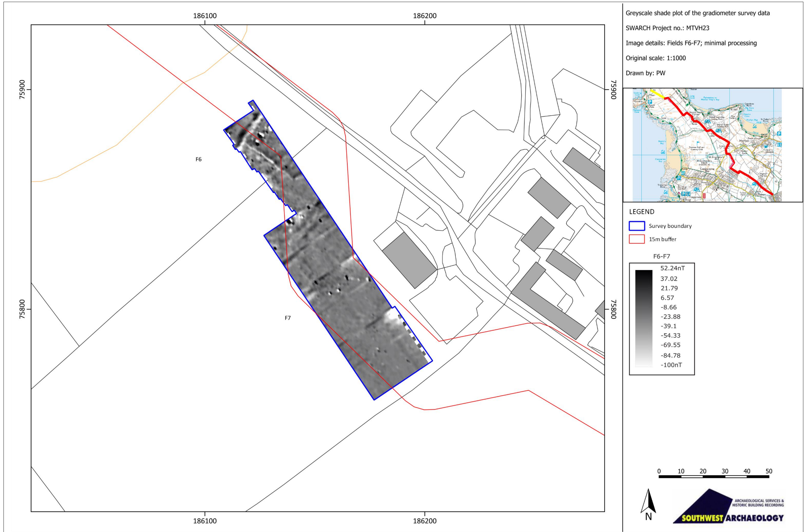
FIGURE 5: GREYSCALE SHADE PLOT OF THE GRADIOMETER SURVEY DATA (FIELDS F6-F7); MINIMAL PROCESSING (CONTAINS ORDNANCE SURVEY DATA © CROWN COPYRIGHT 2023. LICENCE NUMBER 100022432).
