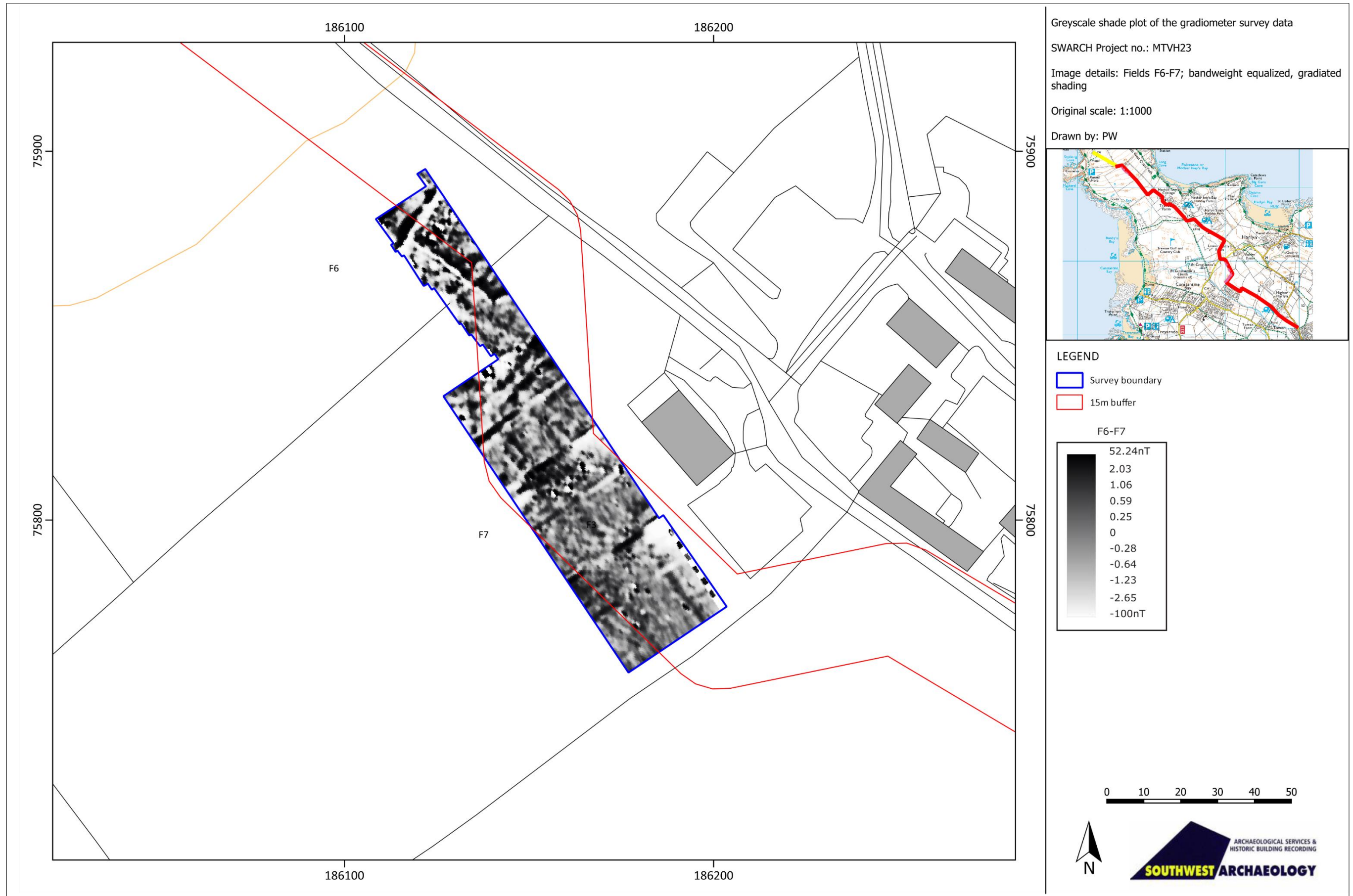
4. GREYSCALE SHADE PLOT OF GRADIOMETER SURVEY DATA (FIELDS F6-F7); BANDWEIGHT EQUALIZED, GRADIATED SHADING (CONTAINS ORDNANCE SURVEY DATA © CROWN COPYRIGHT 2023. LICENCE NUMBER 100022432).
