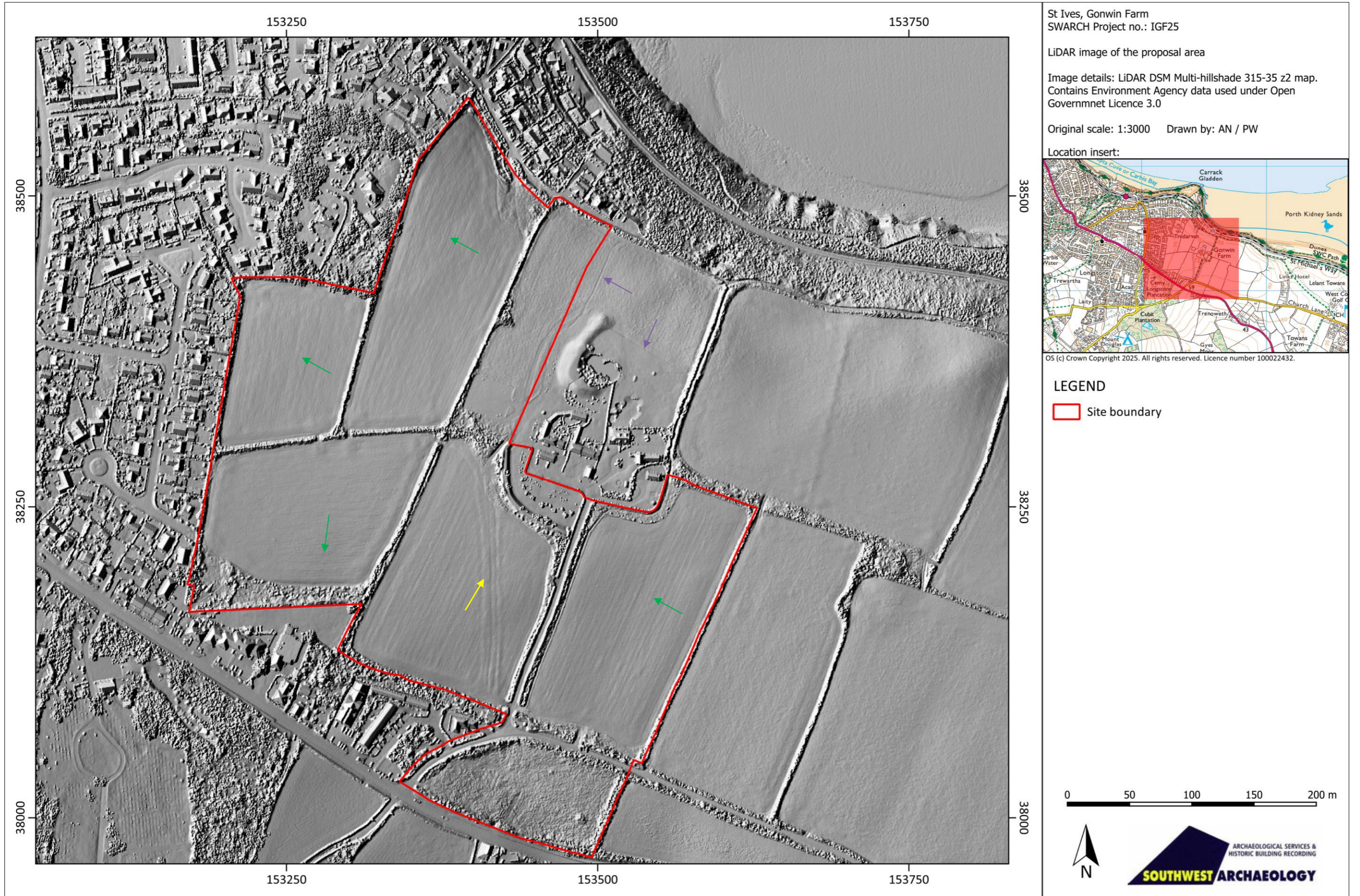
FIGURE 9: 0.50M LiDAR DSM FIRST RETURN DATA. PROCESSED USING QGIS 3.34 MULTI-HILLSHADE 315_35_Z2 SHOWING EXAMPLES OF AGRICULTURAL ACTIVITY (GREEN), HISTORIC BOUNDARIES (PURPLE) AND ACCESS TRACK (YELLOW). CONTAINS ENVIRONMENT AGENCY DATA USED UNDER OPEN GOVERNMENT LICENCE 3.0.
