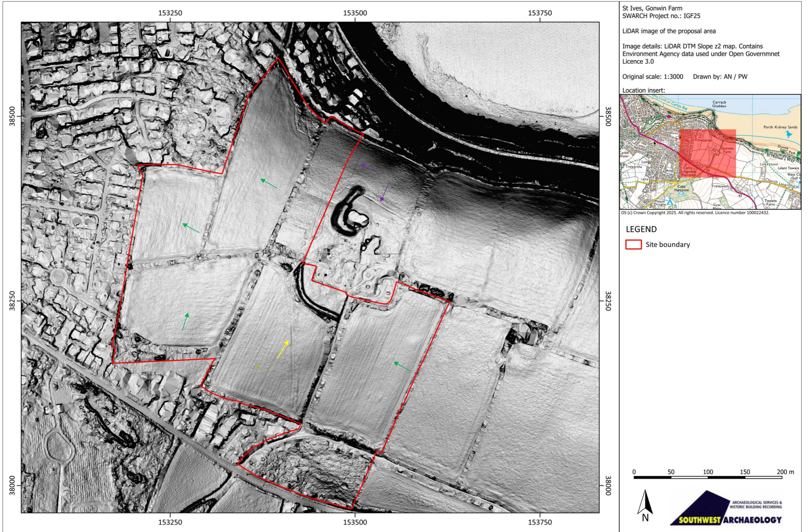
FIGURE 10: 0.50M LiDAR DTM FIRST RETURN DATA. PROCESSED USING QGIS 3.34 SLOPE_Z2 SHOWING EXAMPLES OF AGRICULTURAL ACTIVITY (GREEN), HISTORIC BOUNDARIES (PURPLE) AND ACCESS TRACK (YELLOW). CONTAINS ENVIRONMENT AGENCY DATA USED UNDER OPEN GOVERNMENT LICENCE 3.0.
