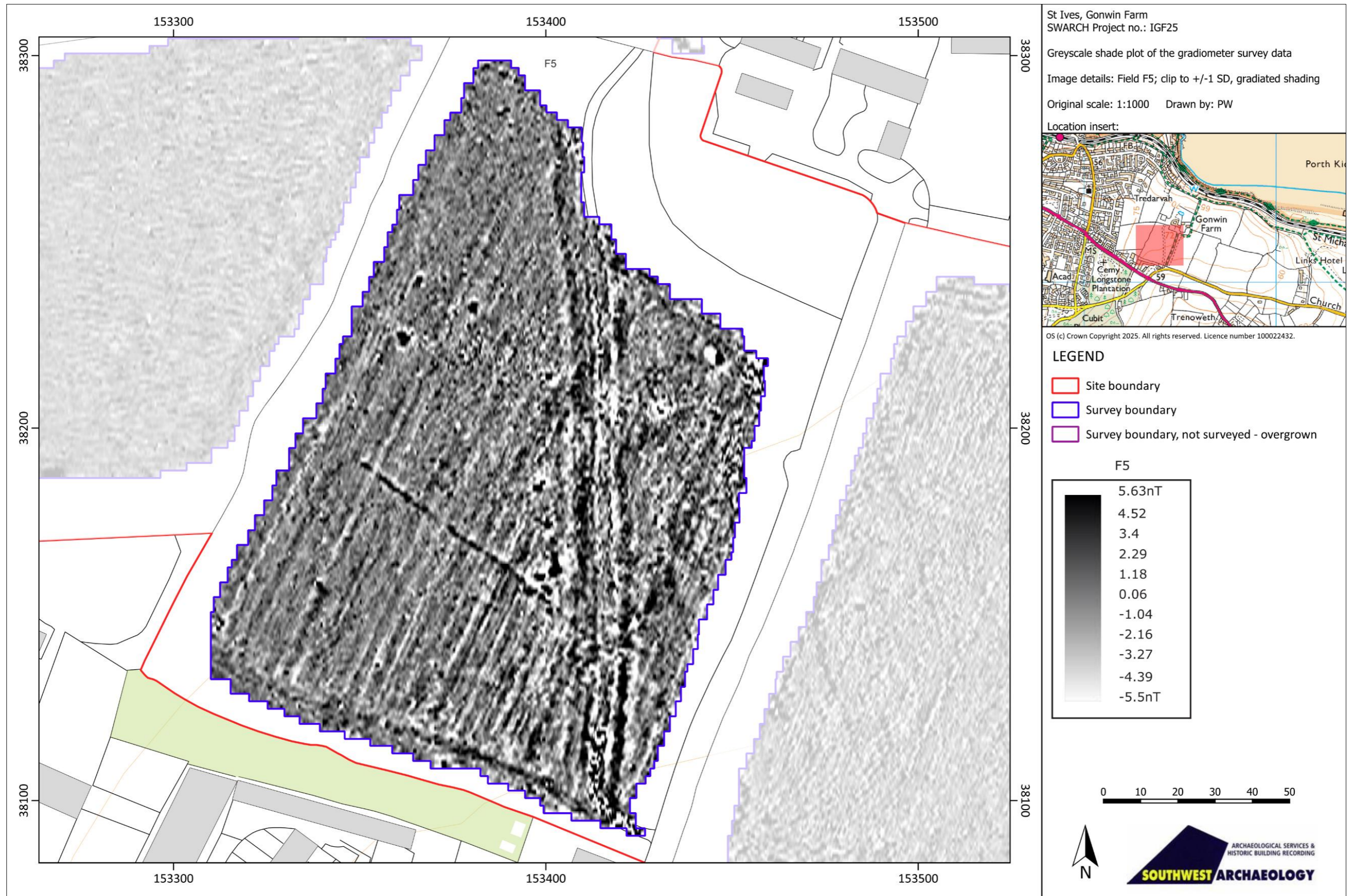
12. FIELD F5, GREYSCALE SHADE PLOT OF GRADIOMETER SURVEY DATA; CLIP TO +/-1SD, GRADIATED SHADING. (CONTAINS ORDNANCE SURVEY DATA © CROWN COPYRIGHT 2025. LICENCE NUMBER 100022432).
