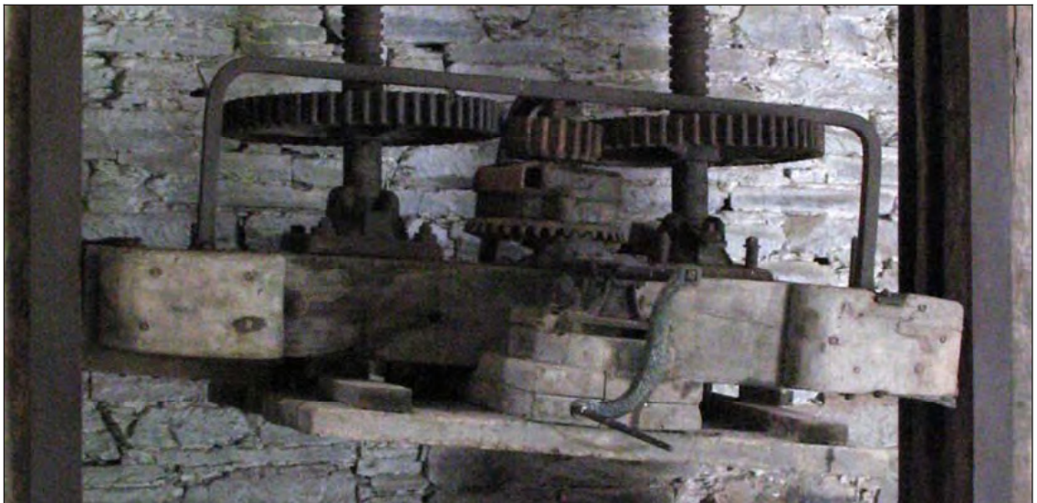
Figure 22: An example of a similar cider press mechanism (crown wheel and pinion) from a press at Buckland Abbey (photo: B. Morris).
