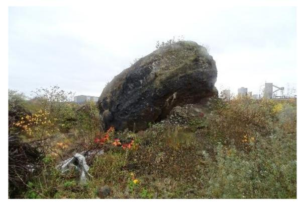
Figure 22: Dislodged plug or salamander from base of Blast Furnace
