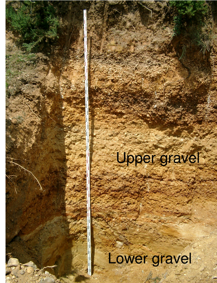
Figure 19. Lepe Country Park sequences, Stone Point. A: estuarine silts and brackish water peats. B: gravels in the cliff adjacent to the beach showing the Upper and Lower gravels.
