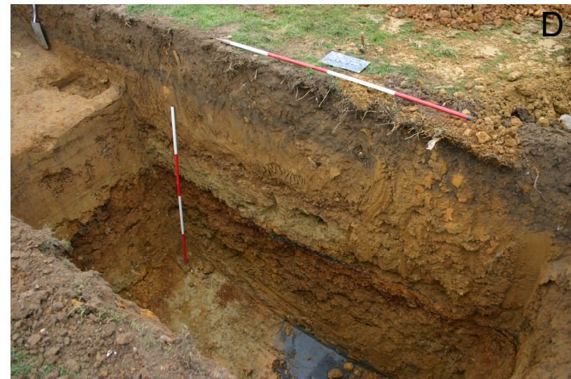
Figure 38. Survey methodology used in PASHCC project. A: Open section recording. B: Terrier drilling. C: Electrical geophysical surveying. D: Test pitting.
