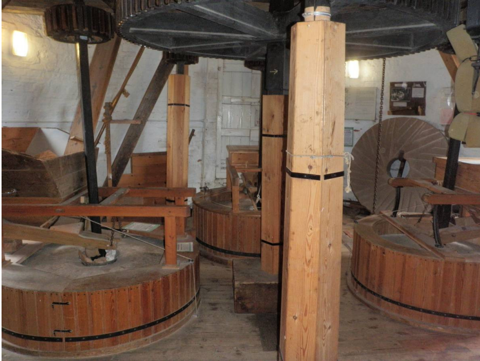
Plate 7. The stone floor showing the three sets of millstones and one of the double access doors, at the rear, on to the external reefing stage
