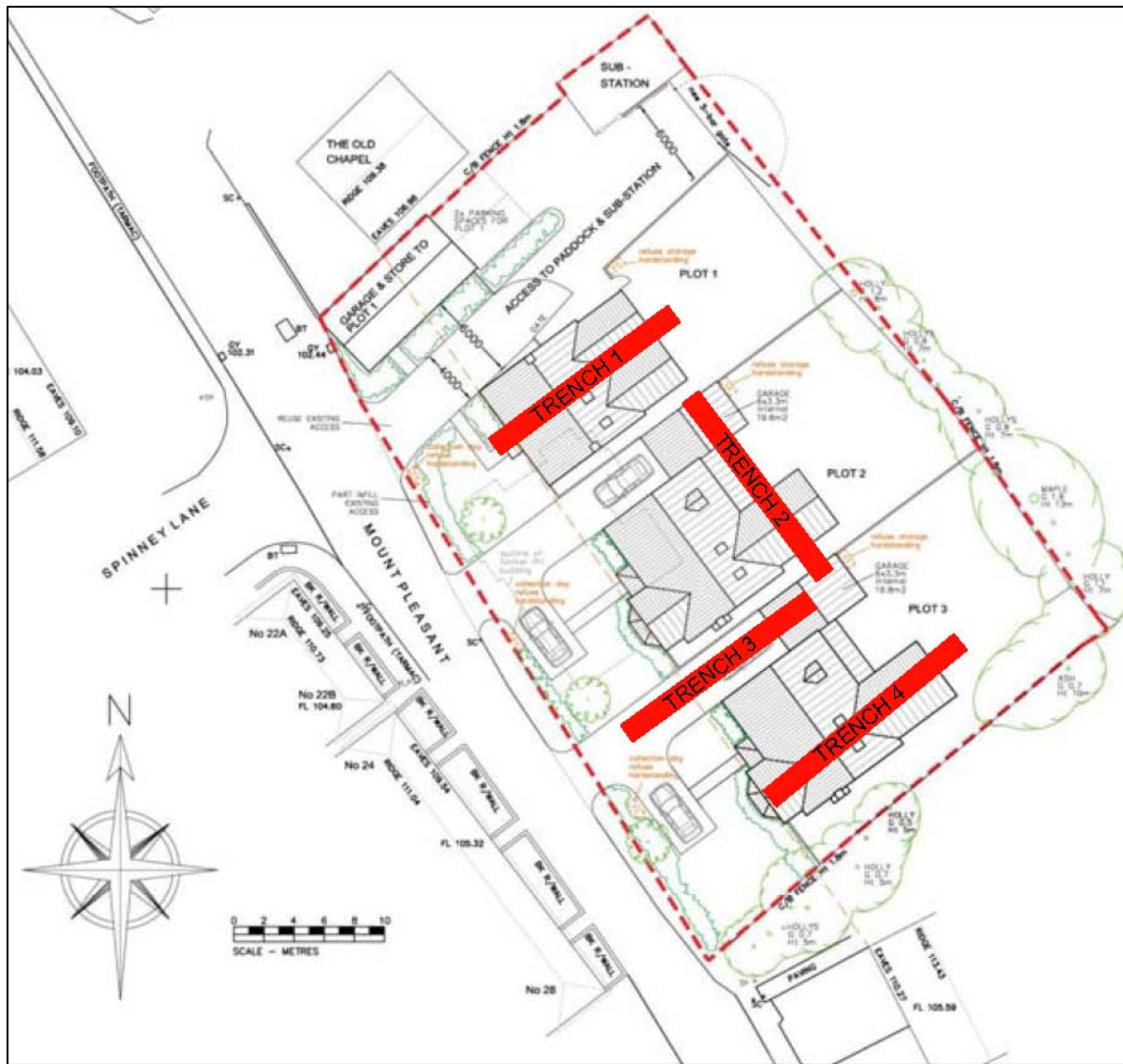
Figure 3: Trench locations (Scale 1:500)
