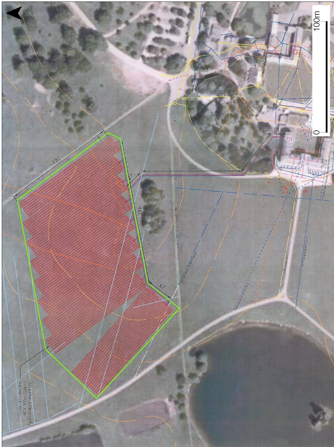
Figure 2: Proposed ground source heat pump pipe array (red) and superimposed geophysical survey area (green) (scale 1:3000)
