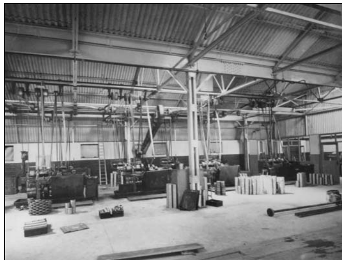
Plate 29: The Automatic Shop. 30 th June 1942. Temporary belt driven Gridley machinery visible in centre
