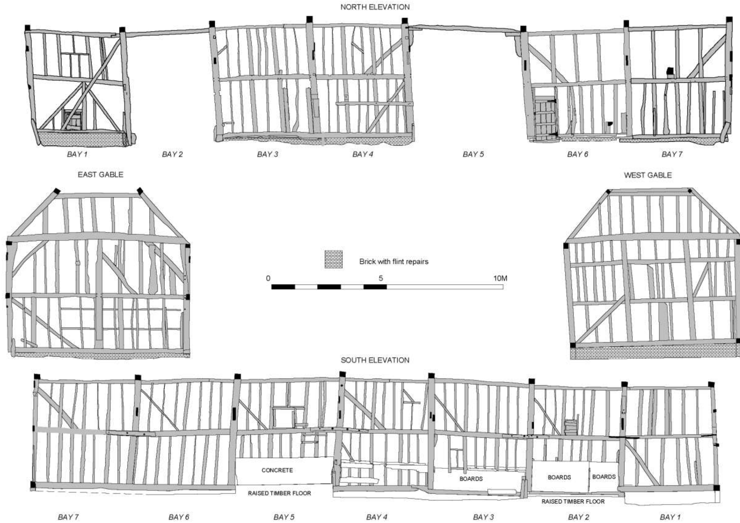
Figure 3: Main barn elevations (scale 1:100)
