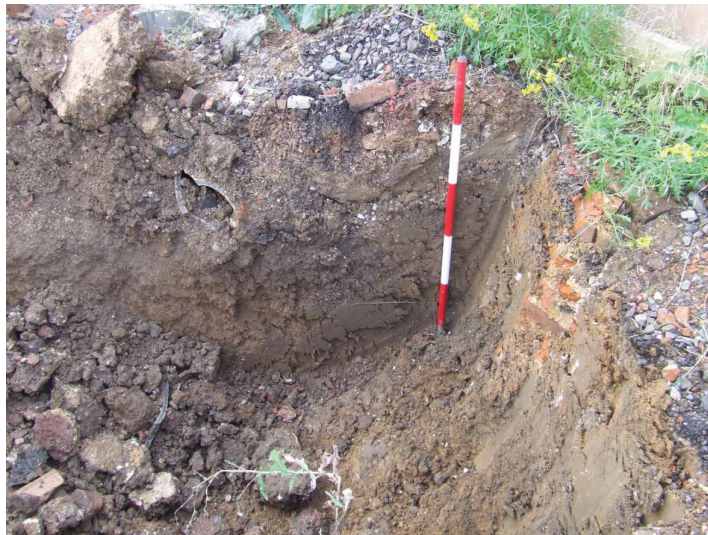
Plate 3: typical test pit section
