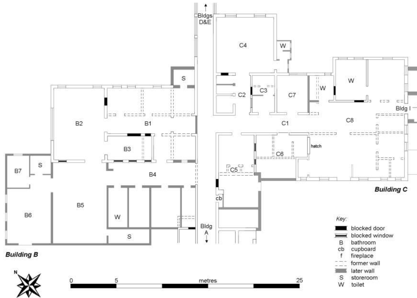
Figure 11: Main hospital block: Buildings B & C (scale 1:200)
