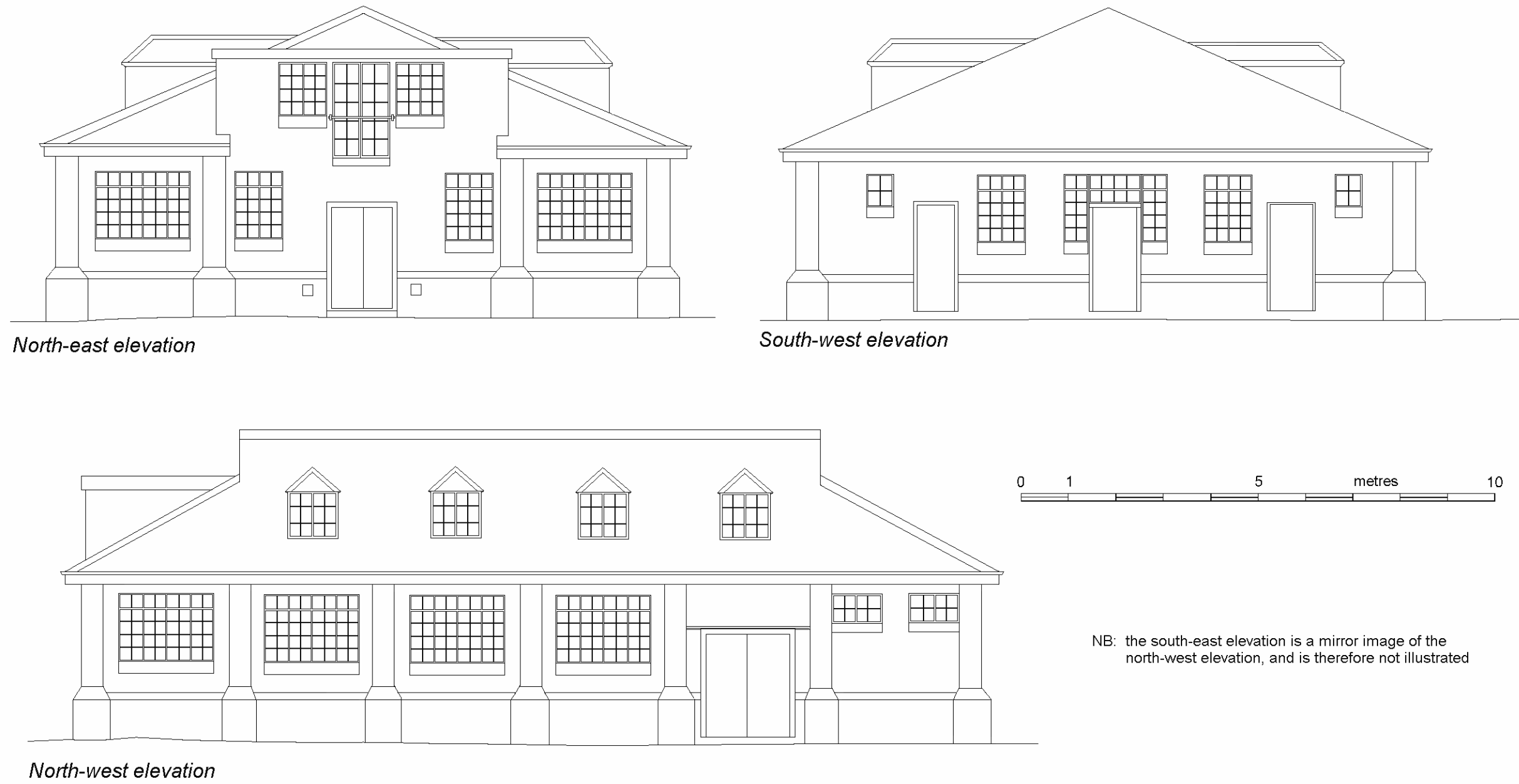
Figure 9: Nursery elevations (scale 1:100)
