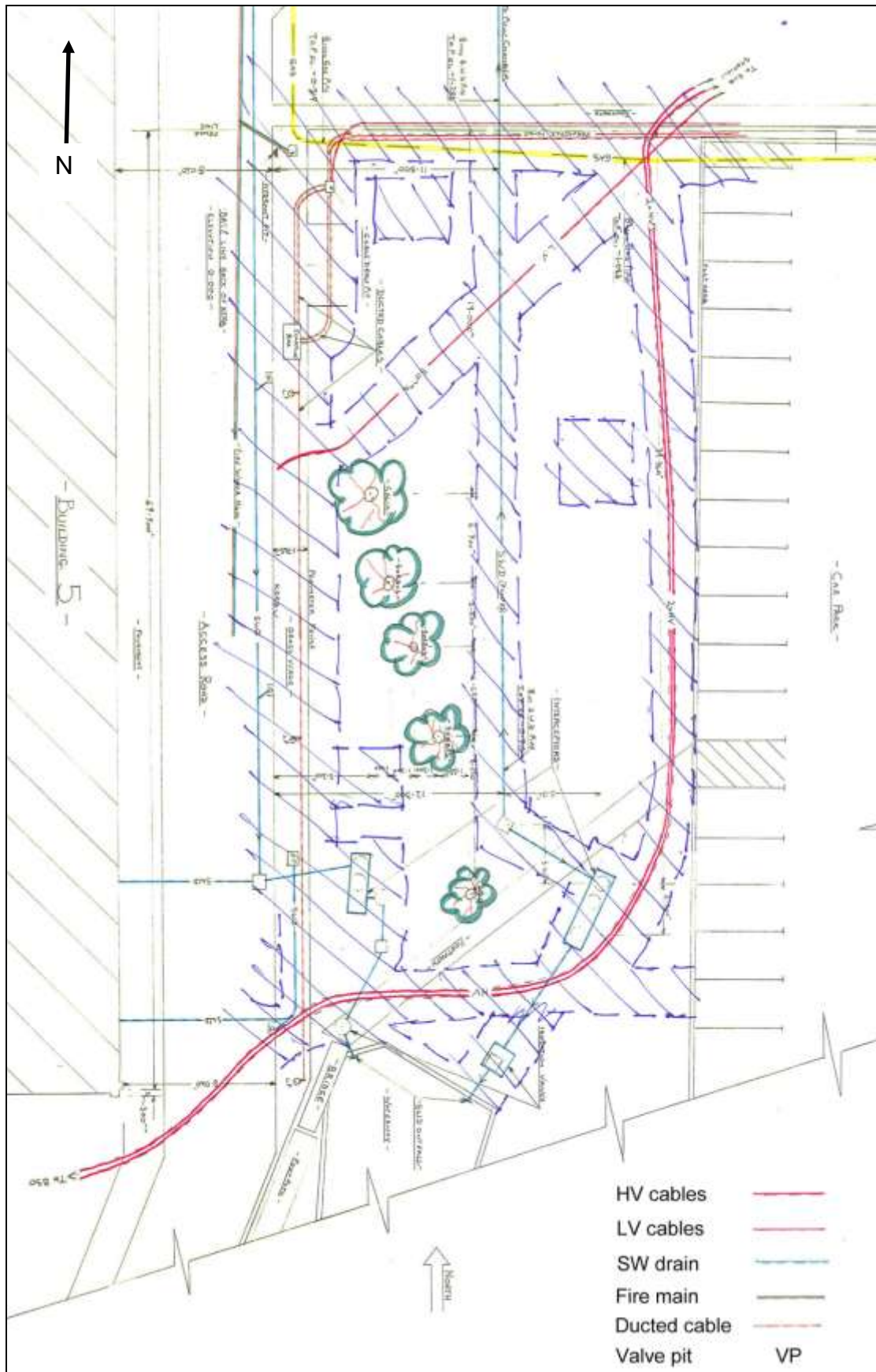
Figure 5: Buried services and other modern disturbances on the site ( not to scale )
