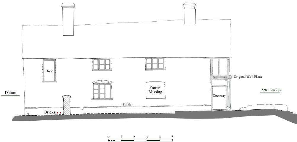
Figure 14: East elevation of the house showing the collapsed south wall
