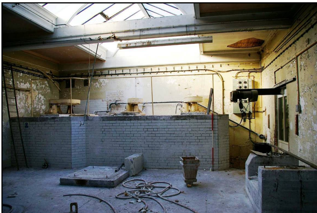
Figure 48: Raised platform with blungers on the west end of the first floor
