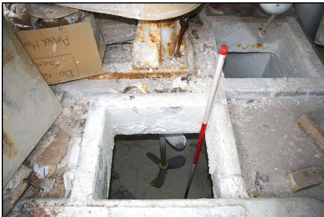
Figure 27: Slip blunger with rotary propeller inside an underground ark
