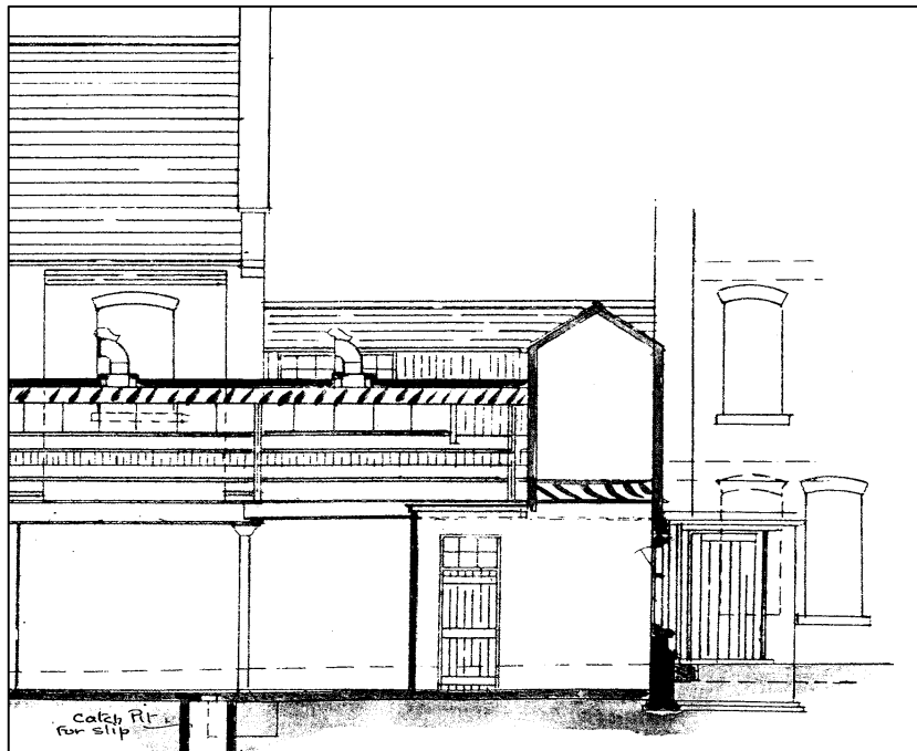
Figure 18: The landing into Building S between Buildings S (left) and R (right). To the front lies the dipping house (Building O) with the bridge at the west end of it running from Building M. 19
