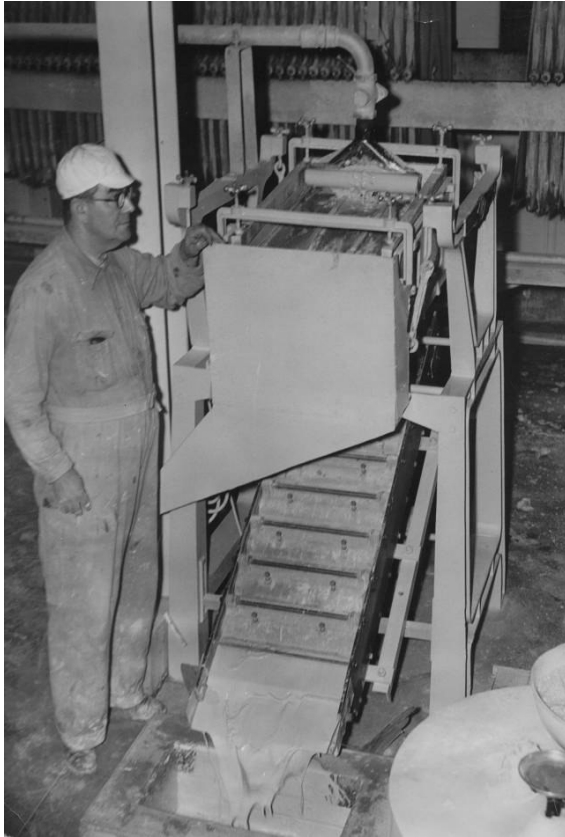
Figure 8: By the 20th century removal of any metallic particles from the liquid clay was done electromagnetically (source: Worcester Porcelain Museum)
