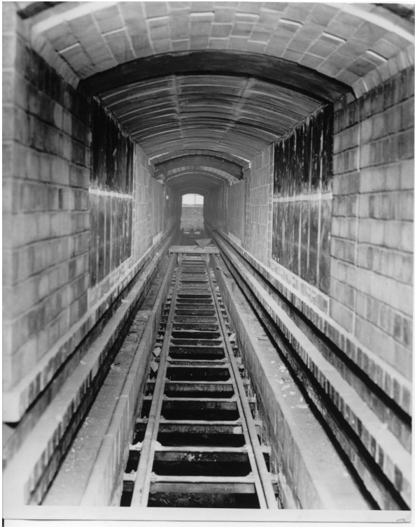
Figure 42: The interior of the Reidhammer kiln. Fire bricks were constantly replaced (source: Worcester Porcelain Museum).
