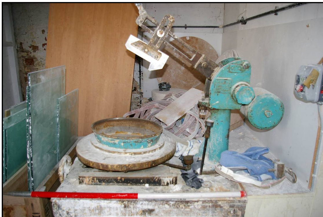
Figure 11: A jolly, used to produce hollow ware
