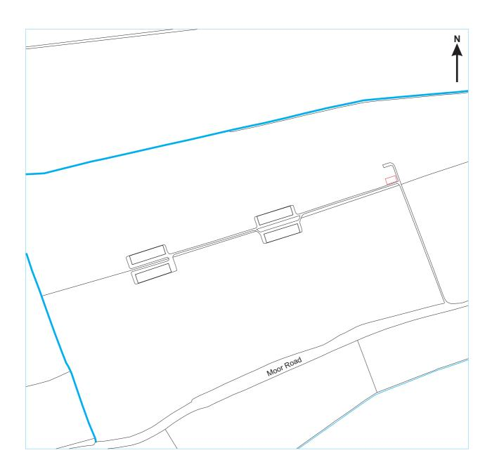
**Figure 2:** Site location, showing the new barn in red, in relation to the new access road and chicken sheds (scale 1:5000)
