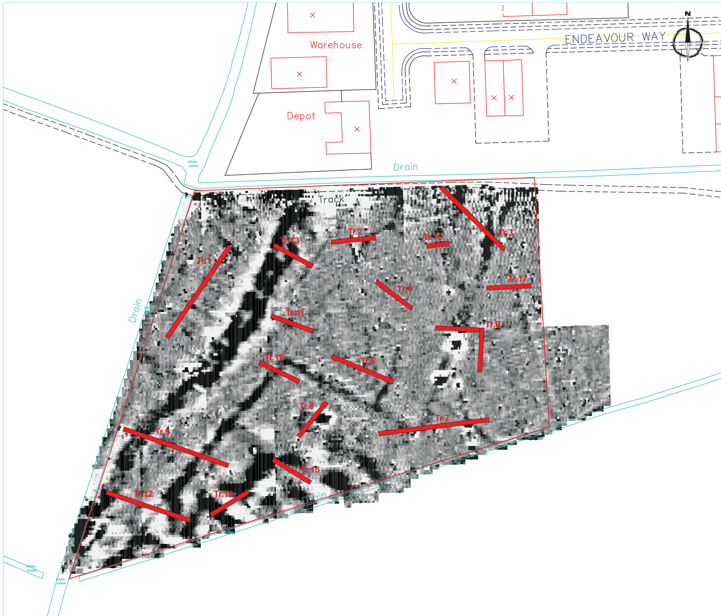
Figure 2: Trench location plan, with trenches in red superimposed on greyscale plan of the geophysical survey at scale 1:1000
