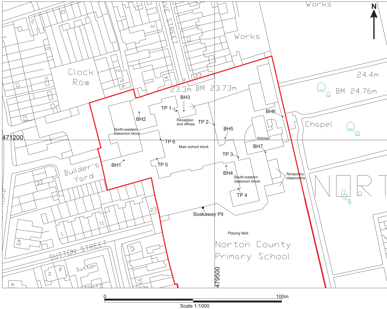
Figure 3: Site plan, showing location of Soakaway Pit, Test Pits (TP) and Boreholes (BH) at scale 1:1000
