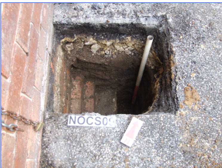
Plate 3: Test Pit 2, south-south-east facing section, looking north-north-west, showing sand layer 201 below bedding layer 200, with natural sand 202 at the base of the sequence.
