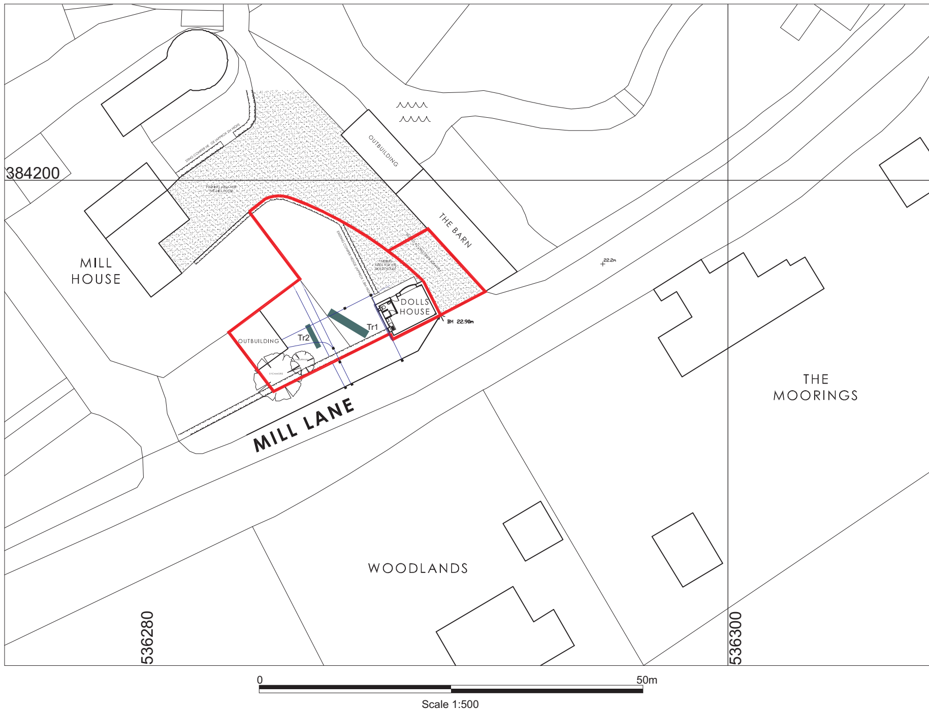
Figure 2: Trench location plan at scale 1:500 showing modern services in blue and evaluation trenches in green
