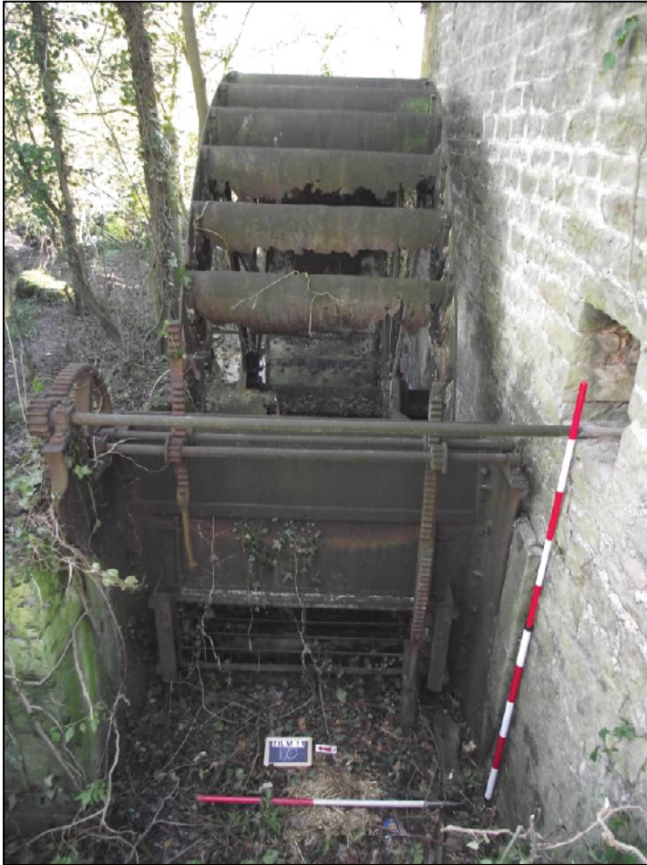
Plate 9 (Shot 10): Detail of the waterwheel and feed tank. Note the horizontal shaft leading into the mill where the control lever for the sluice is situated. The metal bars at the bottom of the tank would sieve the water, keeping the buckets clear from any larger object that could cause damage to the wheel. Looking east
