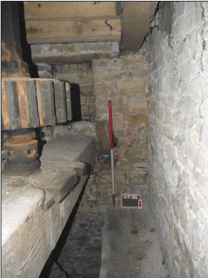
Plate 24 (Shot 51): Stone nut east of the great spur wheel, fitted with an iron spindle which rotates the millstone above (Plate 25). Looking north
