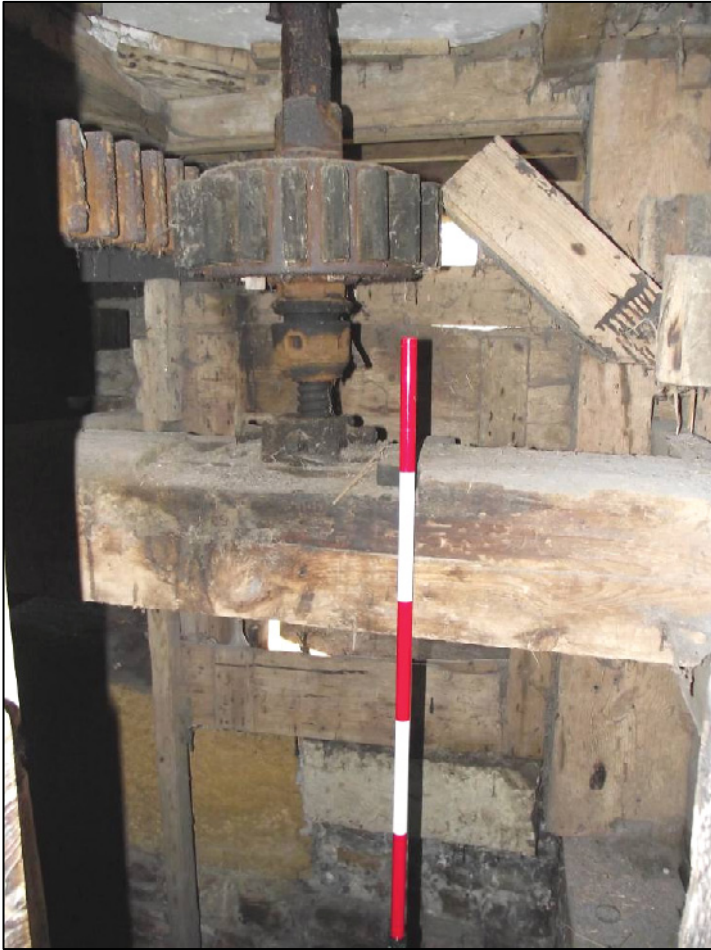
Plate 23 (Shot 45): The horizontal stone nut of iron and wood south of the great spur wheel, sits on a wooden frame and via the iron spindle turns the millstone on the first floor (Plate 25). The flour would then seep through and fall into the wooden chute to the right, into a sack on the outside of the cog-house (Plate 15). Looking east
