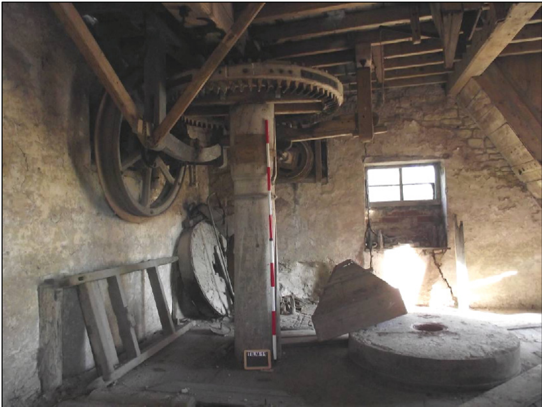
Plate 26: (Shot 53): General shot of machinery on first floor. Note the wooden hopper with shoe (also seen on Plates 25 and 27) on top of the millstone and the horse leaning against the wall, left of the main shaft. Looking east-north-east
