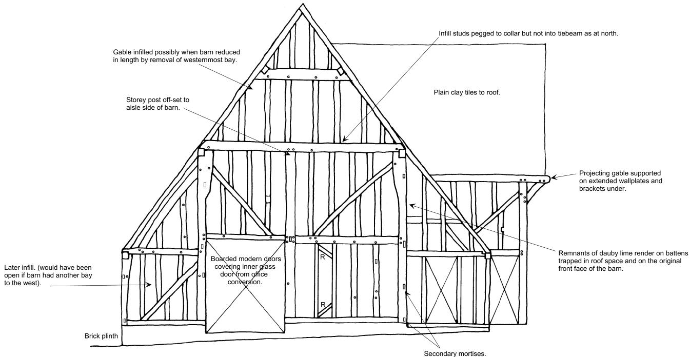
Main details added to outline shape from customer drawings. No detail frame survey available. All timber positions sketched in.
