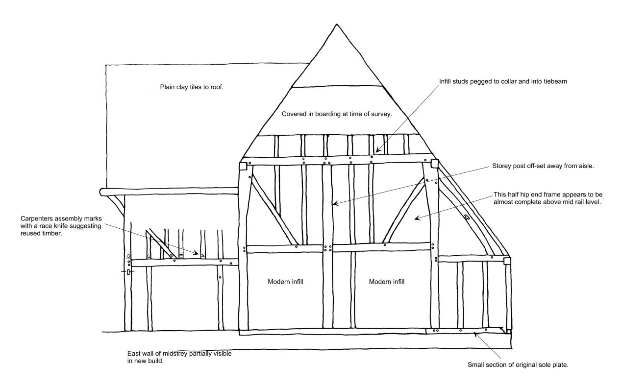
Main details added to outline shape from customer drawings. No detail frame survey available. All timber positions sketched in.
