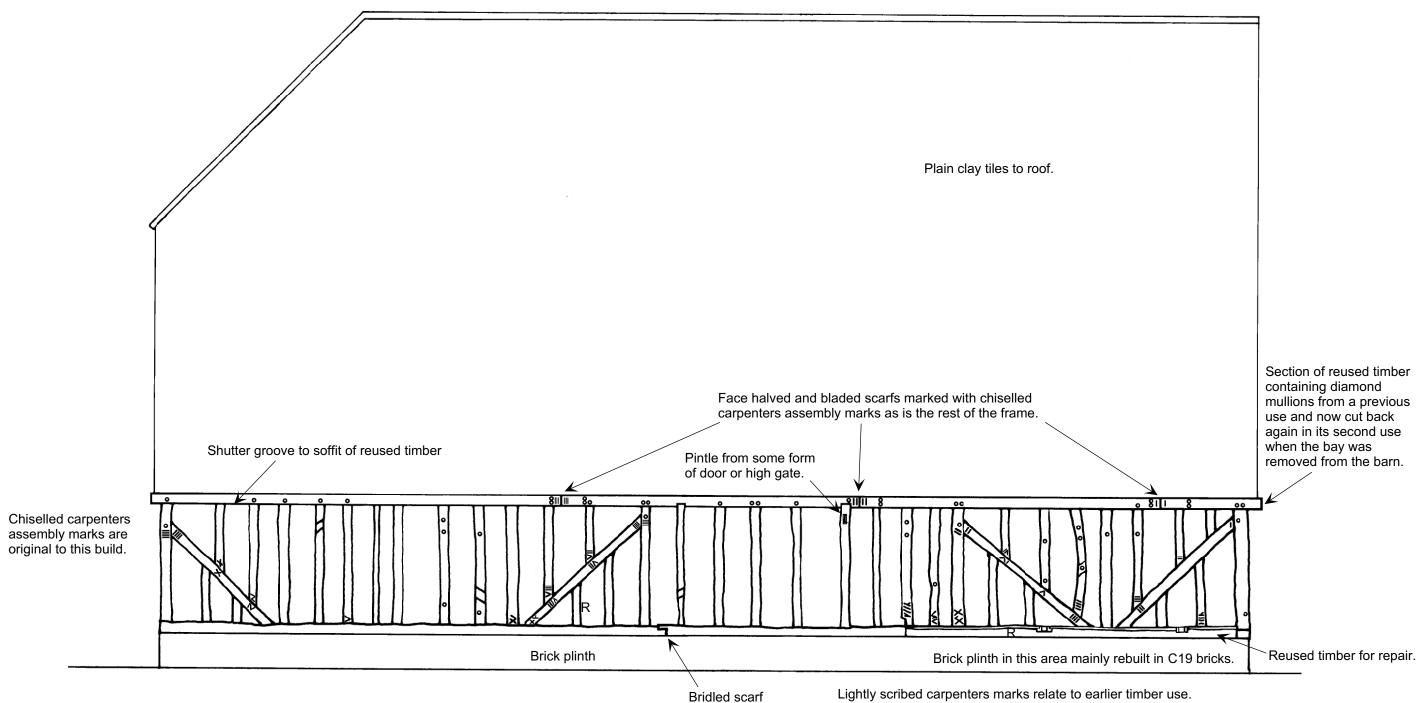
Main details added to outline shape from customer drawings. No detail frame survey available. All timber positions sketched in.
