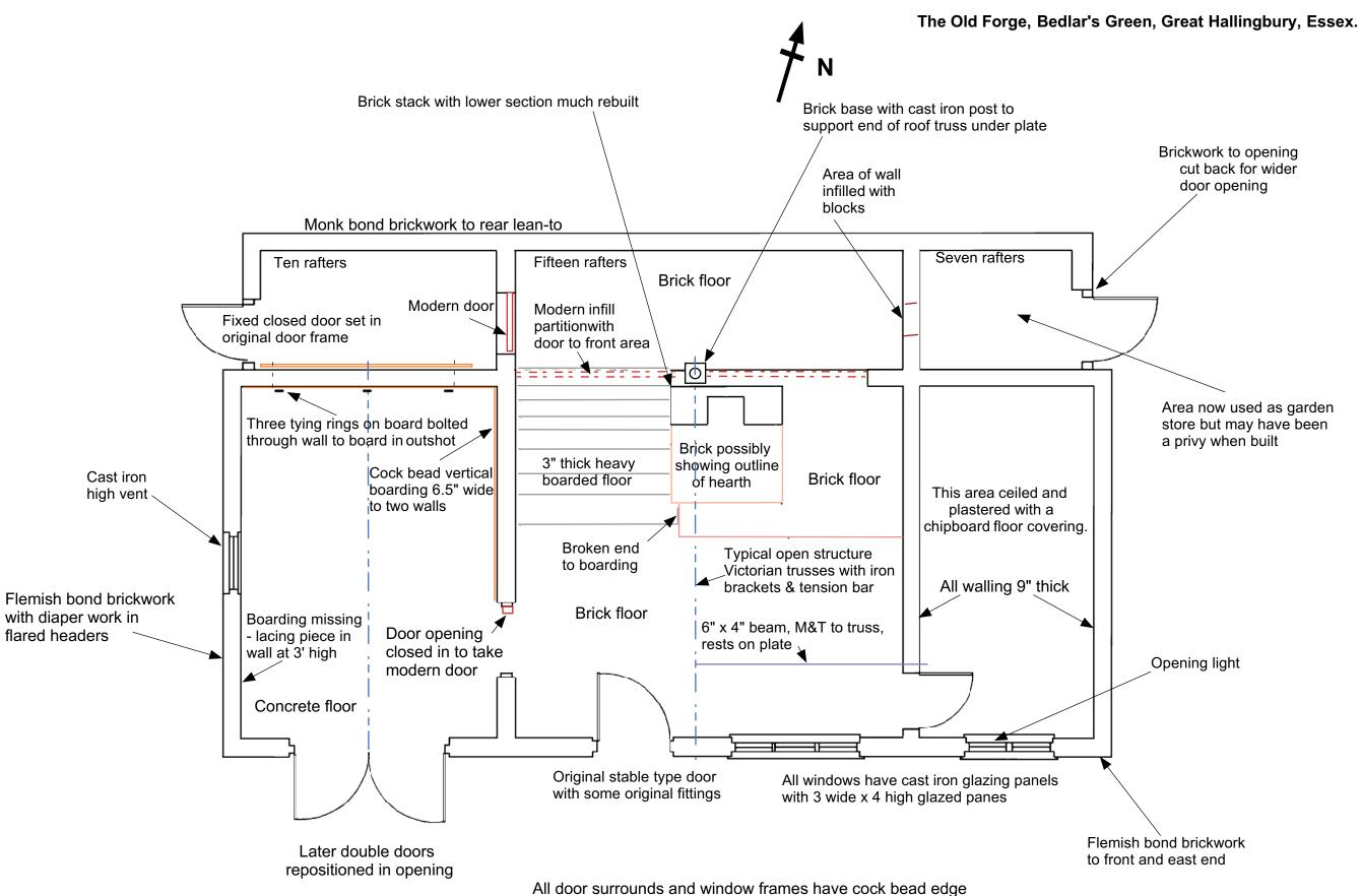
and doors were originally pintle hung. M&T joints with wooden peg.
