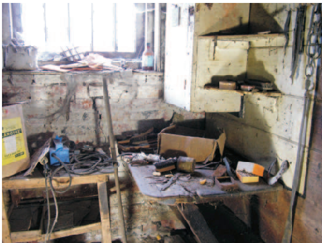
22.CNV The southern end under the window has a timber work bench braced back to the wall.
