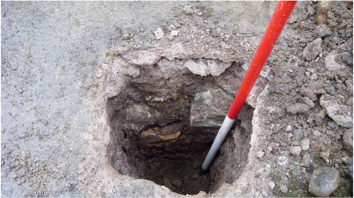
Plate 4: View of hand-inspection pit for borehole showing concrete surface 1029 with underlying rubble deposits 1030 and 1032
