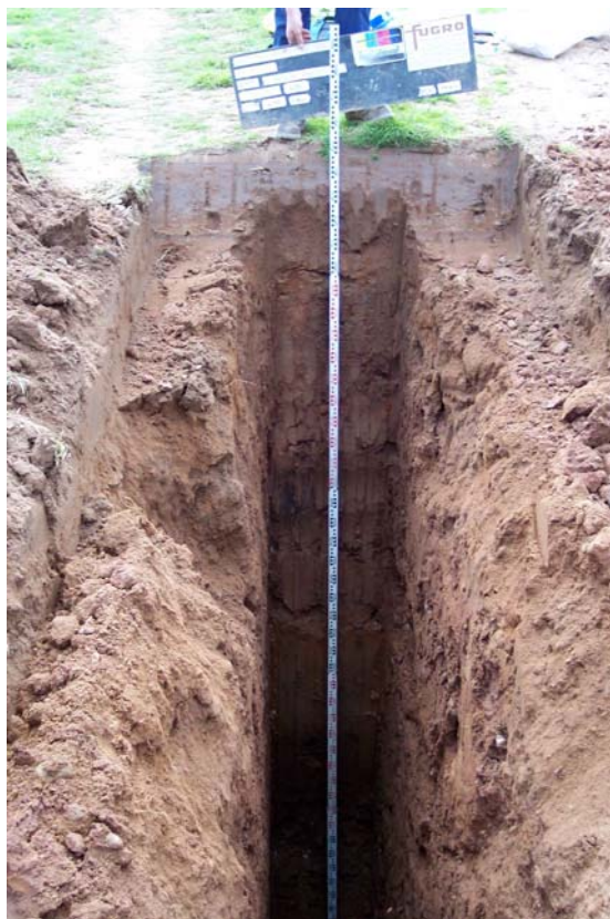
Plate 3: Example of Geotechnical Inspection Pit
