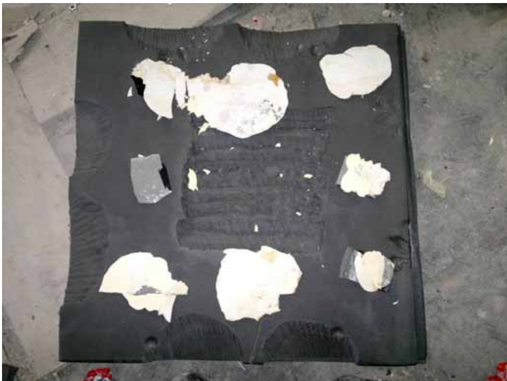
Plate 7: Removed foam piece showing adhered paint and self adhesive tape
