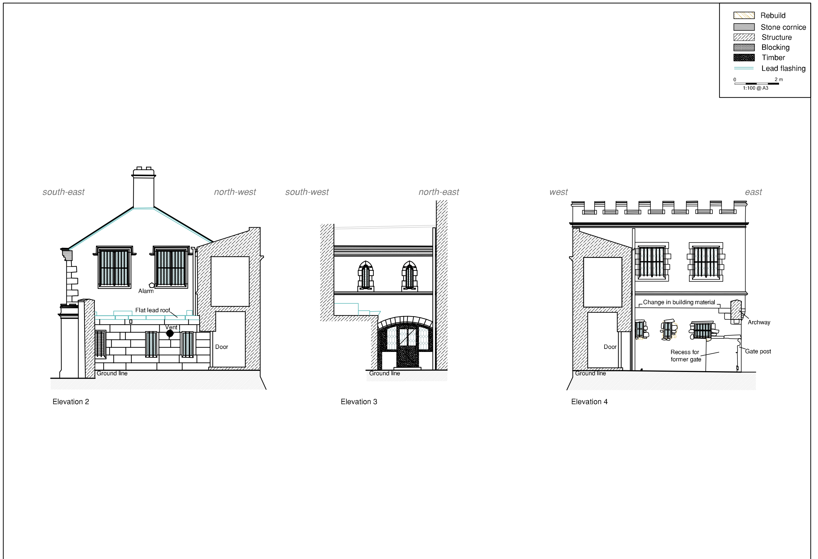
Figure 13: Clitheroe Castle north-, west- and south-facing elevations of the Court House (elevations 2, 3 and 4)
