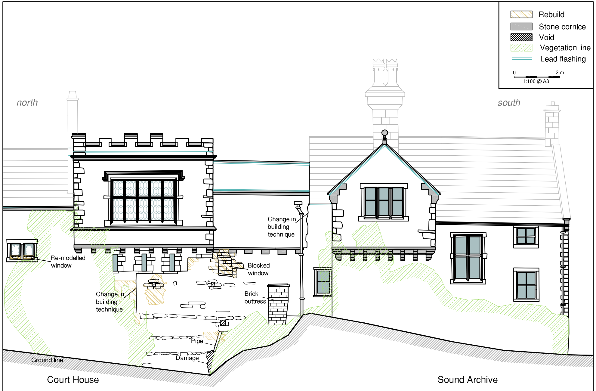
Figure 14: Clitheroe Castle west-facing elevation of the Court House/ Sound Archive (elevation 7)
