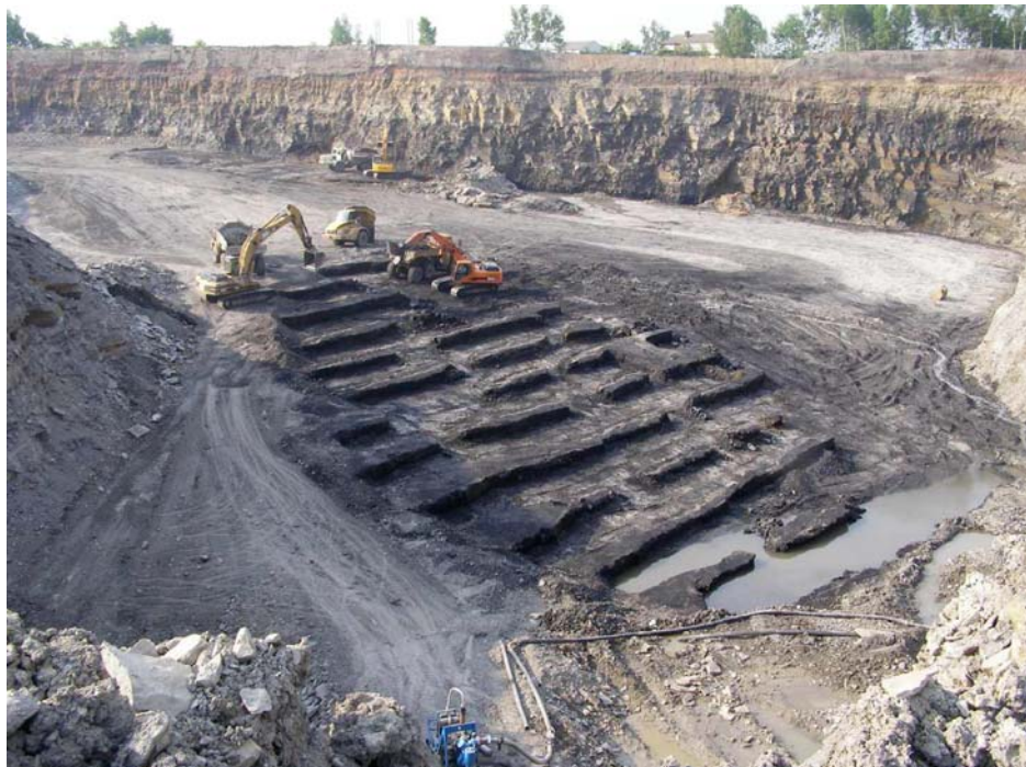
Plate 19: Bord-and-pillar workings uncovered in Area C1
