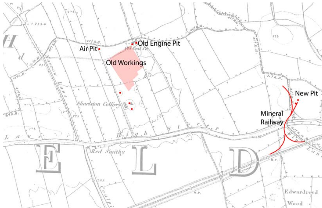
Plate 5: Extract from the 1849 OS 6 inch to 1 mile map, with the locations of the pit-shafts, mineral railway, and ‘old workings’ highlighted, as derived from Greaves’ 1861 plans of the Lower Bed (Sharlston Low Seam)
