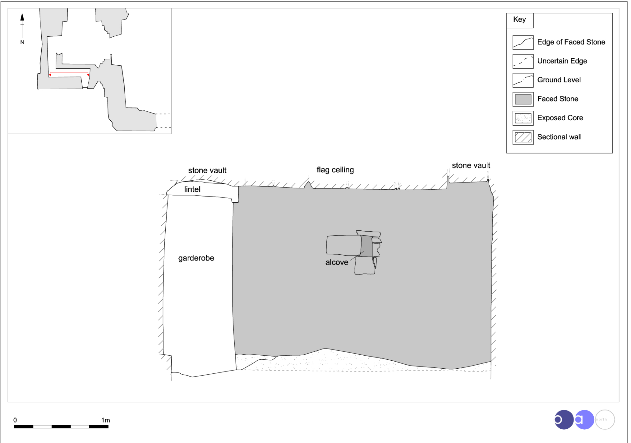
Figure 19: North-facing internal elevation of the barbican garderobe
