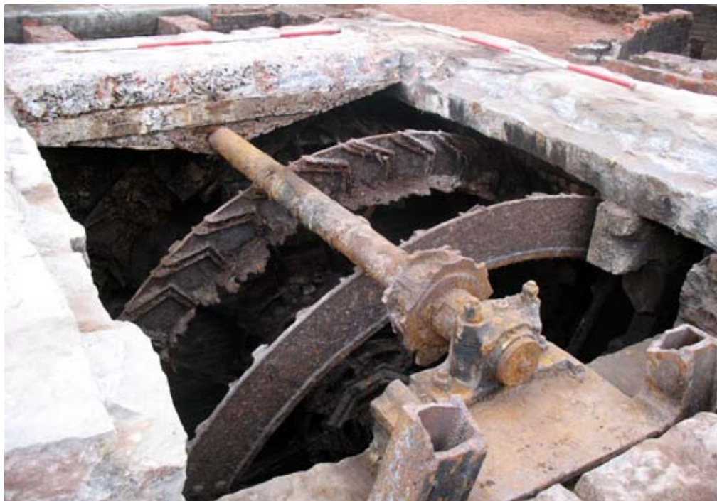
Plate 34: Waterwheel 27 and driveshaft 29 across the top
