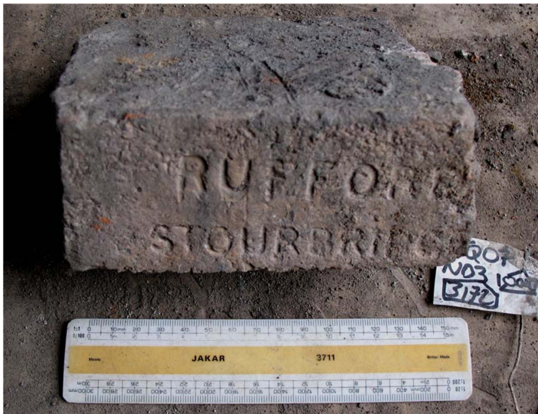
Plate 21: Sample of a refractory brick manufactured by Rufford & Co of Stourbridge
