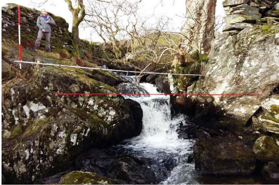
Plate 5 – The proposed location for the intake structure photographed during the design process, the horizontal red line represents the height of the proposed intake structure.
