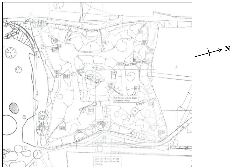
Figure 8: Contour plan of the Queen's Sconce earthwork (not to scale), showing the erosion scars to be repaired.
