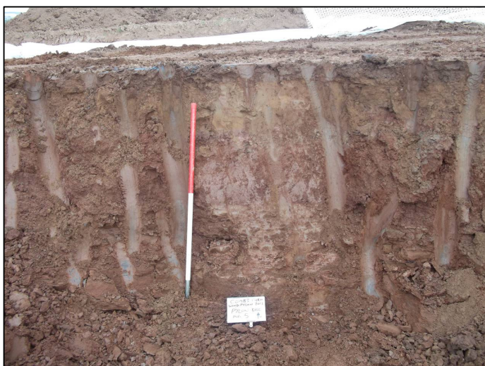
Plate 3: Sample section at safe working depth in the pylon base pit, looking N, showing the sequence of natural deposits.
